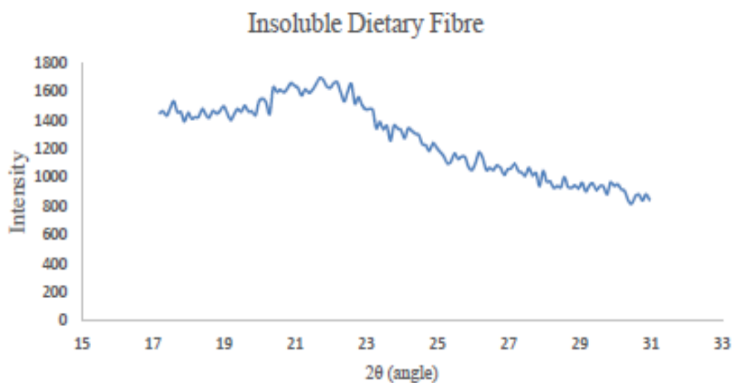
Fig.2.13 X-ray powder diffraction (XRD) pattern of insoluble dietary fibre (IDF)
